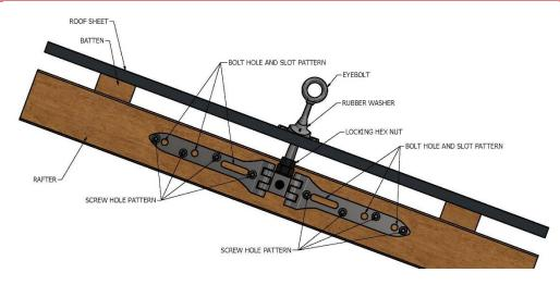
The HingeLink is designed for use on timber structures where there is easy access to the underside of the roof.
